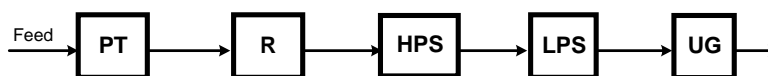
Fig. 1. Flow sheet of the HTU process. PT: pre-treatment; R: reactor; HPS: high-pressure separator; LPS: low-pressure separator; UG: upgrading unit.
